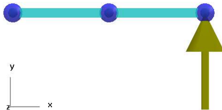
Figure 3.30: 3 point masses are constrained to each other with MultiCoordConstraints to obtain the same behaviour as a rigid body, see the provided example code.
